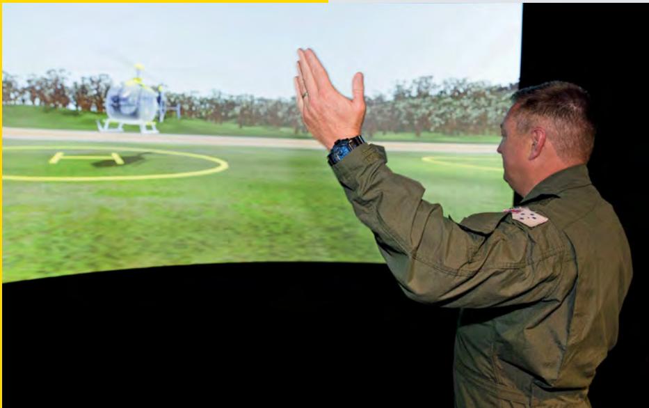
An aircrewman uses the flight marshalling synthetic training equipment of the Helicopter Advanced Training System at HMAS Nowra. Cpl Mark Doran/Australian Army
