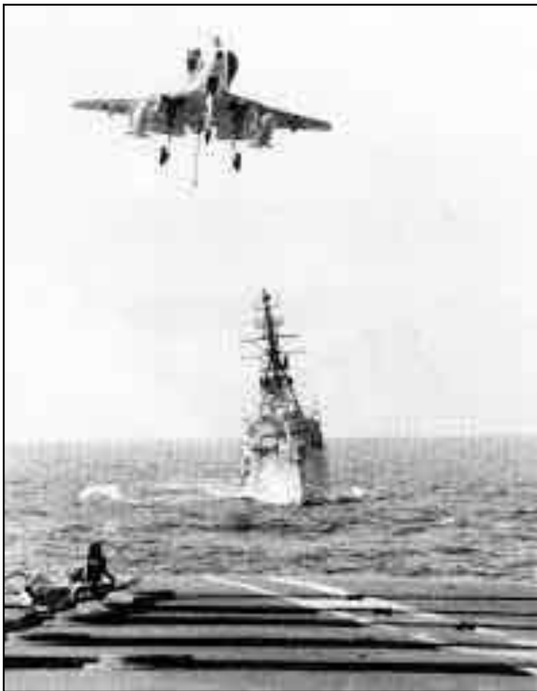
A4 on short final (hook down) preparing to trap whilst DDG astern acts as 'plane guard' (SAR)
