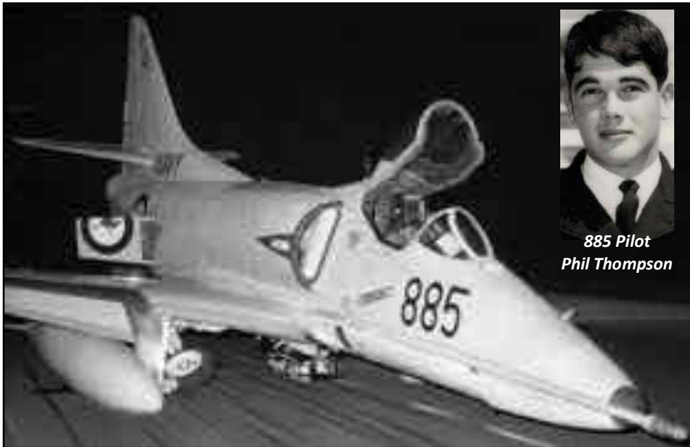
A4 885 after an arrested landing back at NAS Nowra on drop tanks. Note: The collapsed main undercarriage after the ramp strike!
