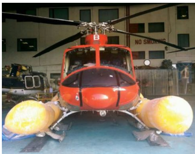
A civilian Bell 412 with flotation gear deployed.
