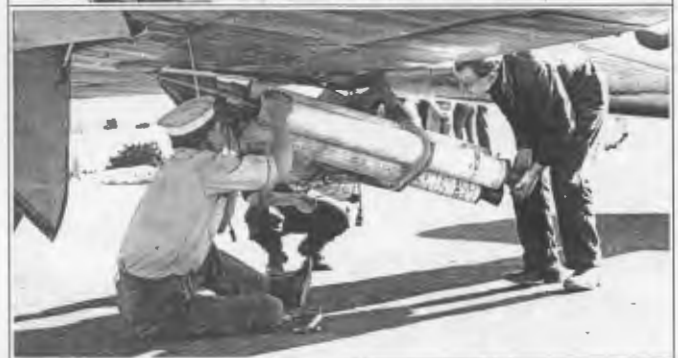
JERVIS BAY AIRFIELD 1950 Armourers assembling and fitting RATOG equipment All photographs this page courtesy AMoF
