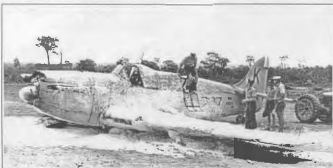
LT LEESON'S FIREFLY CRASH AT RANAS NOWRA The result of a RATOG malfunction and only one side firing Photo courtesy AMoF
