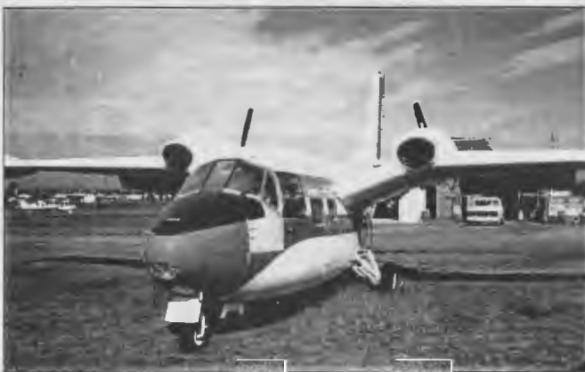
Italy's uniquely configure Piaggio P166 was used extensively by Australian regional airlines. VH-MMP, which arrived at the museum in May, was used for many years by MacRobertson - Miller airlines in West Australia. (AMoF)
