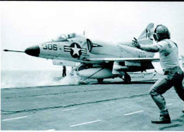
A VA 154 A-4 Skyhawk with two big 1000 lb bombs and a 400 gallon centreline tank launches from the Midway-Class USS Coral Sea (CV-43) for a North Vietnam target.
