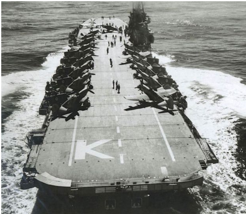
HMAS Sydney's Flight Deck circa 1950/51, showing the 'through deck'. The relative size of the Sea Furies (forward) and Fireflies (aft) give an indication of just how narrow the deck was, and how little room there would have been for stowing aircraft on the deck during flying operations. Image: Allen Porter.
