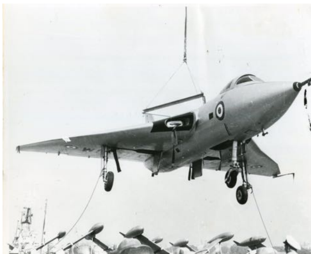
The Avro 707 – a one third size testbed for the Vulcan Bomber – being loaded aboard HMAS Melbourne in 1956.
