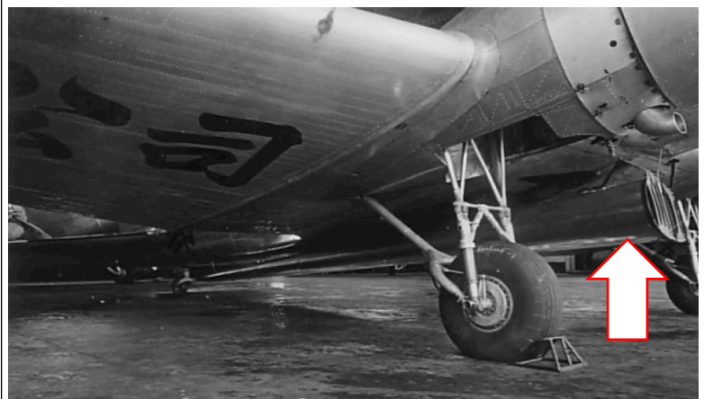
Top: Zygmund Soldinski, CNAC's Chief of Maintenance, posing with the wing section strapped to the underside of the DC2 courier aircraft. The fitting can be seen on the lower image, although the butt fairing is yet to be fitted.
