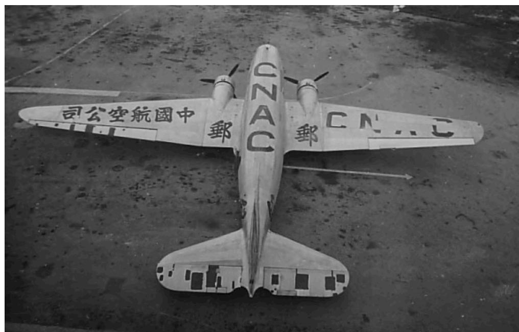
Above. The DC "Two and a Half", as flown out of China. The right wing can be seen to be demonstrably shorter than the left. The story was to add grist to the already widespread belief that the Douglas DC series of aircraft were extraordinary workhorses.
