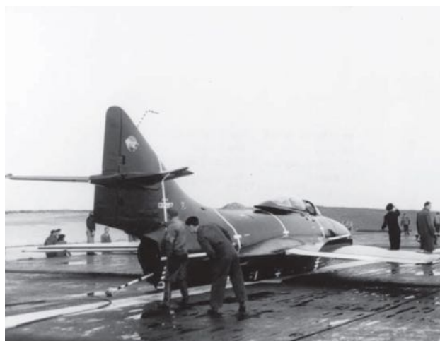
Grumman F9F-7 Cougar (BuNo 130862) upon completion of an arrested landing at NAS Patuxent River on February 1, 1955. The belly of the aircraft was beefed up significantly to absorb landing loads. (NNAM)
