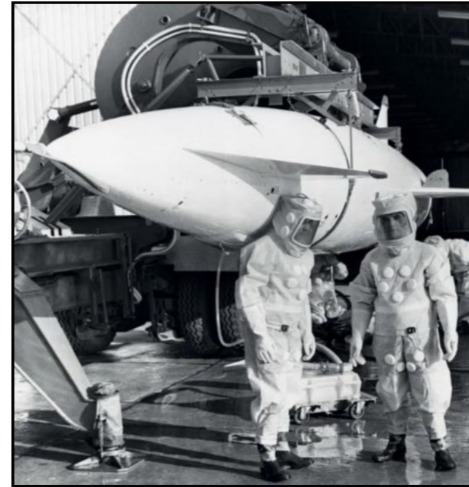
Technicians fuel a Blue Steel Missile. The fuel mixture was highly volatile, requiring full protective clothing and water damping during the process. →
