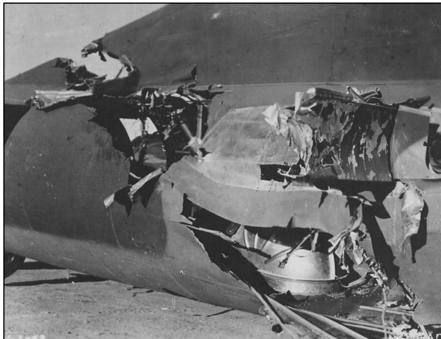
Above and right. Close ups of the damage caused by the German fighter's wing as it struck the aft fuselage of the B17. The structural spars supporting the tail assembly were sufficiently undamaged to hold together, but the entire port stabiliser was missing. Remarkably, none of the crew were injured.
