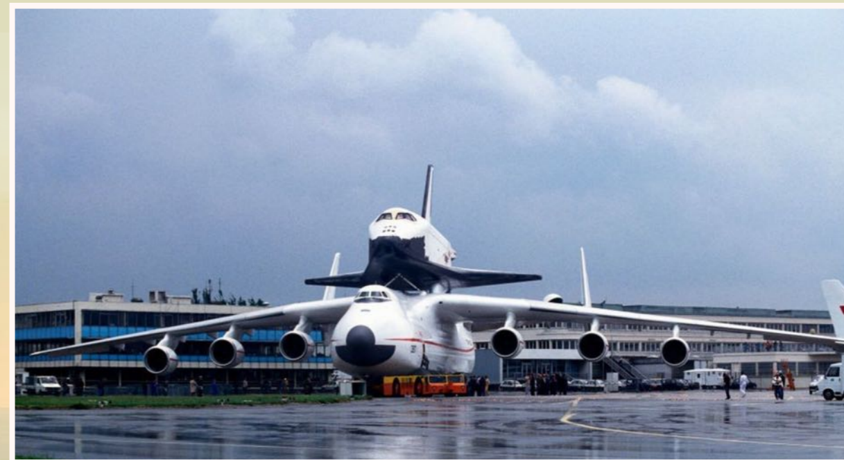
Above. The An-225 "Myira" carrying a Buran Class orbiter on its back. Below. Despite being the world's largest heaviest aircraft at a gross weight of 640 tonnes, the An-225 was remarkably graceful. Only one was ever completed and it was destroyed in 2022, when the Russians invaded Ukraine. ✈
