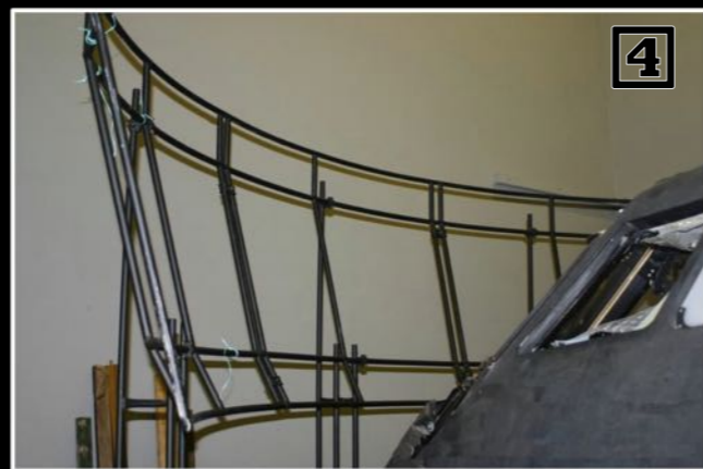
[1] The original simulator under construction at British Airways in 1975. [2] The projection generator: cameras mounted on a moving gantry which scanned over a detailed model of some topography or an image of an airport. [3] The cockpit module being moved to Brooklands. [4] Construction of the frame for the projection screen. [5] The frame was covered by white material, onto which the landscape image was projected [6]. ✈
