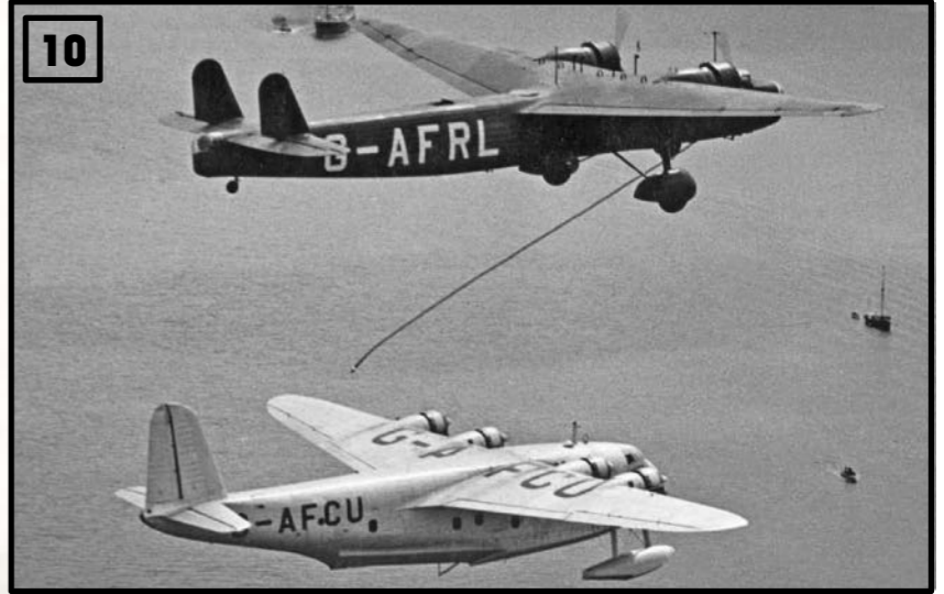
A total of 16 trans-atlantic crossings were made using the "Looped Hose" or "Ejector" method of coupling. ✈
